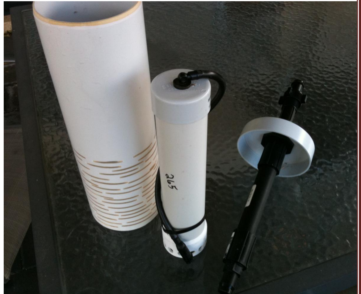
Figure 2 Bell siphons were placed in each growbed. The siphons fasten a 100 mm pipe cap to the base of the Acme tank using a tank tap. The stand tube screws up or down for slight height adjustments and the slotted siphon shield is made of 100 mm drainage pipe.
